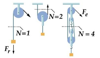
A pulley is a wheel over which a rope or belt is passed. It is also a form of the wheel and axle. Pulleys are often interconnected in order to obtain considerable mechanical advantage. Pulleys may be used to change the direction of the force or to increase the ease of lifting an object.
