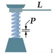
A screw is an inclined plane wrapped in a spiral around a shaft.
