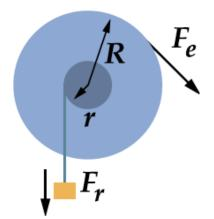
A wheel and axle are essentially a modified lever, but it can move a load farther than a lever can. The center of the axle serves as a fulcrum. Gears, belts, cams, and cranks include applications of a wheel and axle.
