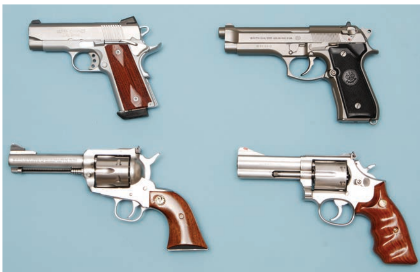
Pistols have many types of actions. Clockwise from top left: single-action semi-automatic, double-action semi-automatic, double-action revolver, and single-action revolver.
