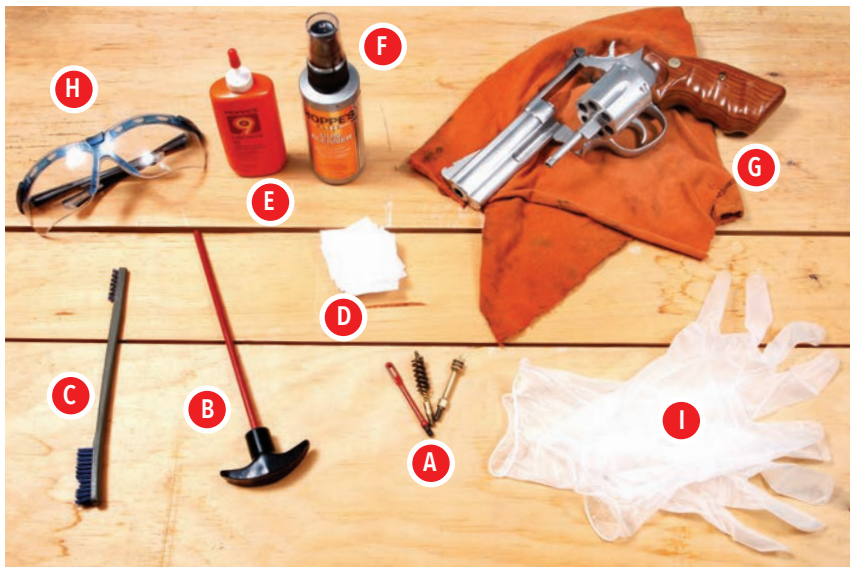
The components of a basic gun cleaning kit, including (A) a bore brush and jags for holding cleaning patches, (B) a cleaning rod, (C) a small brush, (D) cotton cleaning patches, (E) gun oil, (F) gun cleaning solvent, (G) a soft cloth, and (H) eye protection. Also shown are thin rubber gloves (I), which may help protect the skin from dirt, oil, and solvent.
