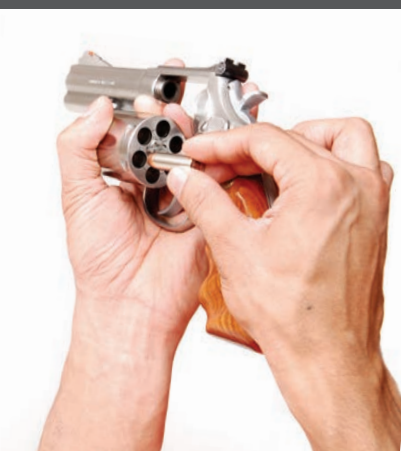
Most single-action revolvers are loaded through a gate in the frame (left). The cylinder of a modern double-action revolver (right) swings out to allow access to all chambers.
