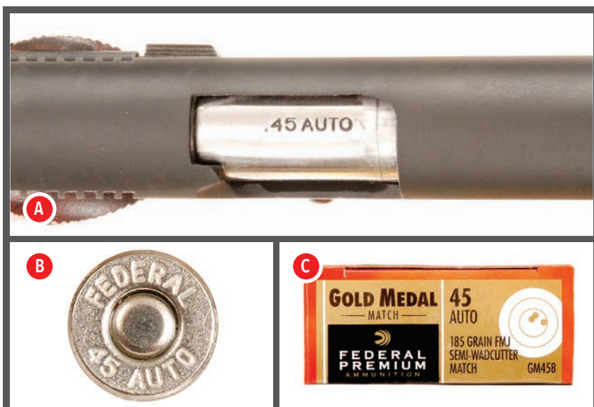
The proper ammunition for a given pistol is determined by matching the markings on the barrel (A) with the cartridge designation on the headstamp (B) and the cartridge box (C).
