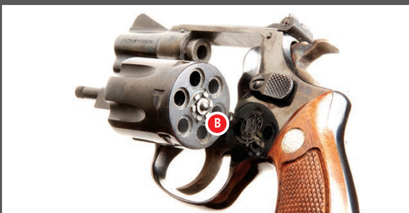
Revolvers are characterized by a rotating cylinder with several chambers. Each time the hammer is cocked (single-action revolver) or the trigger is pulled (double-action revolver), the hand or pawl rises in its window in the recoil shield (A) and engages one of the ratchets on the extractor star (B) of the cylinder, rotating it to the next chamber.
