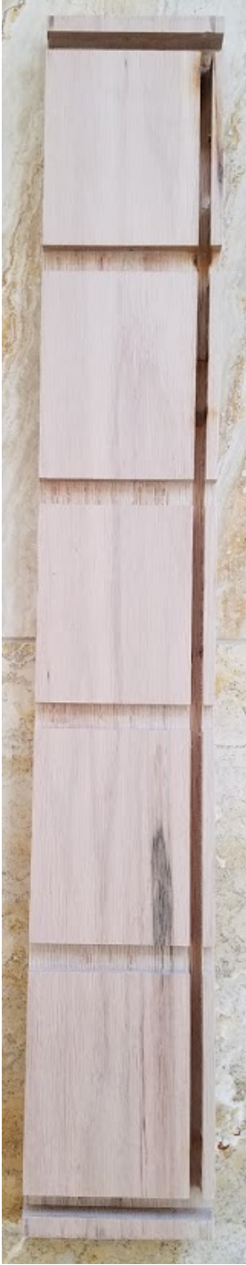
Picture 1 – Cabinet Frame side pieces - Shown with frame cutouts, shelf cutouts and router groove for back panel.
