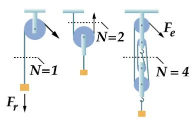
A pulley is a wheel over which a rope or belt is passed. It is also a form of the wheel and axle. Pulleys are often interconnected in order to obtain considerable mechanical advantage. Pulleys may be used to change the direction of the force or to increase the ease of lifting an object.
