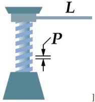
A screw is an inclined plane wrapped in a spiral around a shaft.
