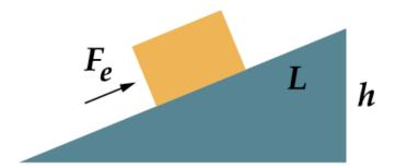
An inclined plane is a device such as a ramp, stair, or ladder and is used to more easily raise a load. The steepness of the incline affects the level of ease of movement. While a shallow incline makes it easier to raise a load, the length of the incline must be longer to compensate.
