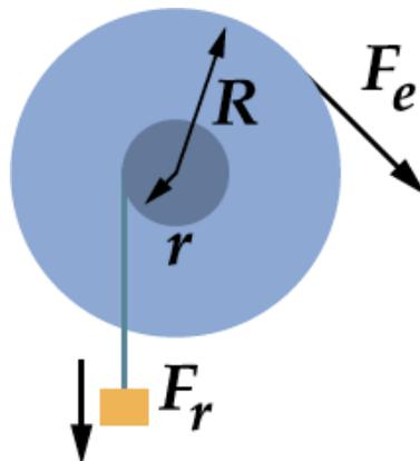
A wheel and axle are essentially a modified lever, but it can move a load farther than a lever can. The center of the axle serves as a fulcrum. Gears, belts, cams, and cranks include applications of a wheel and axle.
