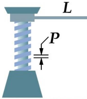
A screw is an inclined plane wrapped in a spiral around a shaft.
