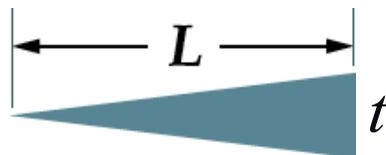
A wedge is a movable double incline plane used to separate objects using force. Examples include a knife, ax, and nail.
