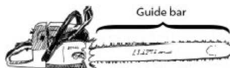
**GUNNING SIGHTS** – Lines on the power head that are perpendicular to the guide bar. Used as a tool to aim the direction in which a tree will fall. When the sights are aimed at the felling lane, the bar will be perpendicular to the felling lane. Remember, the horizontal cut and back cut of the conventional face cut are to be perpendicular to the felling lane.
