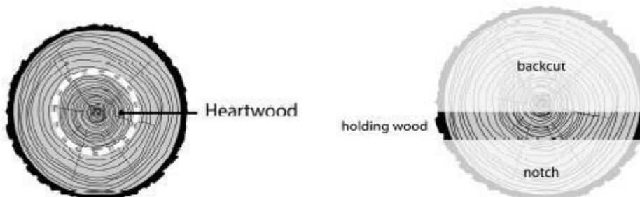
HINGE (aka “holding wood”) – The section of wood not cut in the felling sequence. Its purpose is to guide the falling tree in the desired direction while preventing the tree from coming off the stump until it has been committed to the face. Holding wood thickness should be approximately 10% of DBH (e.g., 1” for a 10” tree). **ALWAYS MAINTAIN THE INTEGRITY OF YOUR HINGE!**
