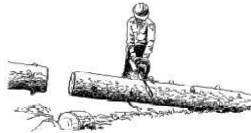
BUTT – The bottom portion of a tree trunk or log; the first bucked portion of a felled tree.
