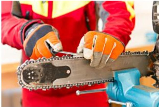
The depth gauge rides on the wood and controls the depth at which the cutting corner bites into the wood.
